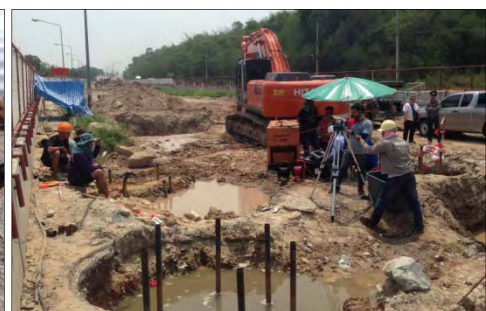
Cross Hole Sonic Logging Test
