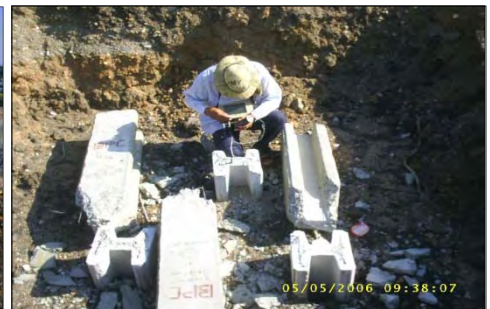
Seismic Testing on Driven Pile
