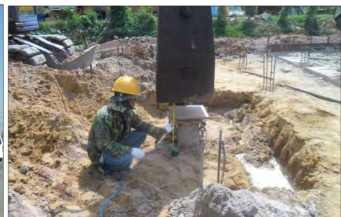
Dynamic Load Testing on Driven pile
