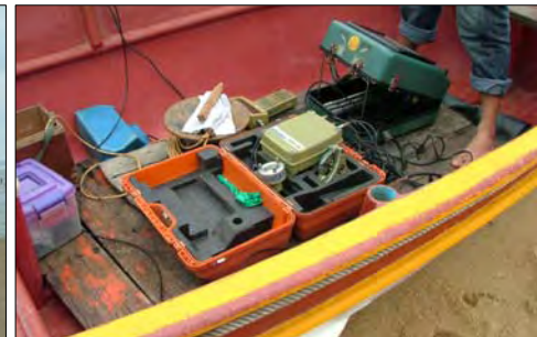
Survey Equipments (GPS &amp; Echo Sounder)
