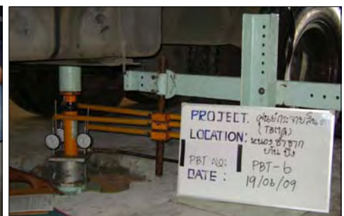
Plate Bearing Test on Ground Support
