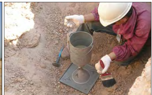
Field Density Testing at TP-4
