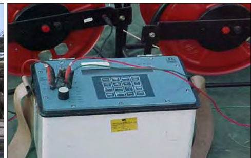
Syscal R1 Plus Resistivity Meter
