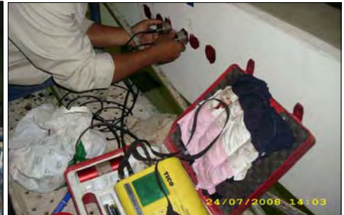
UPV Test at Beam
