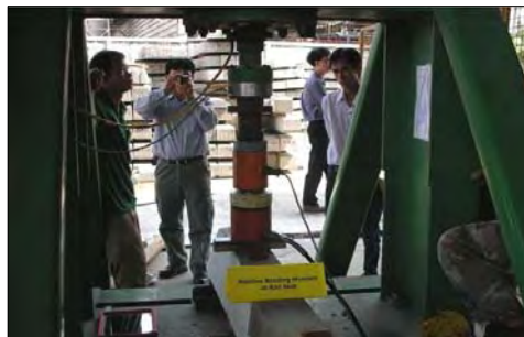
Positive Bending Moment at Rail Seat
