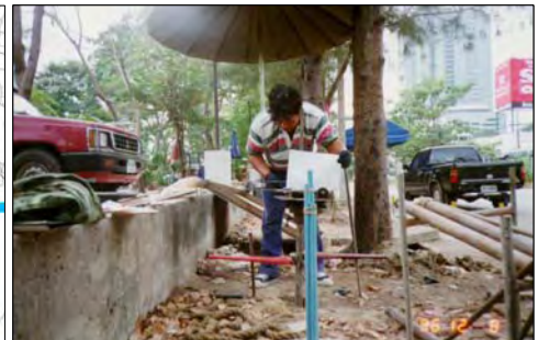
Field Vane Shear Test on Phetchakasem Road
