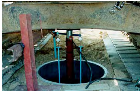
Arrangement for Compressive Load Test
