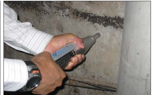
Rebound Hammer Test
